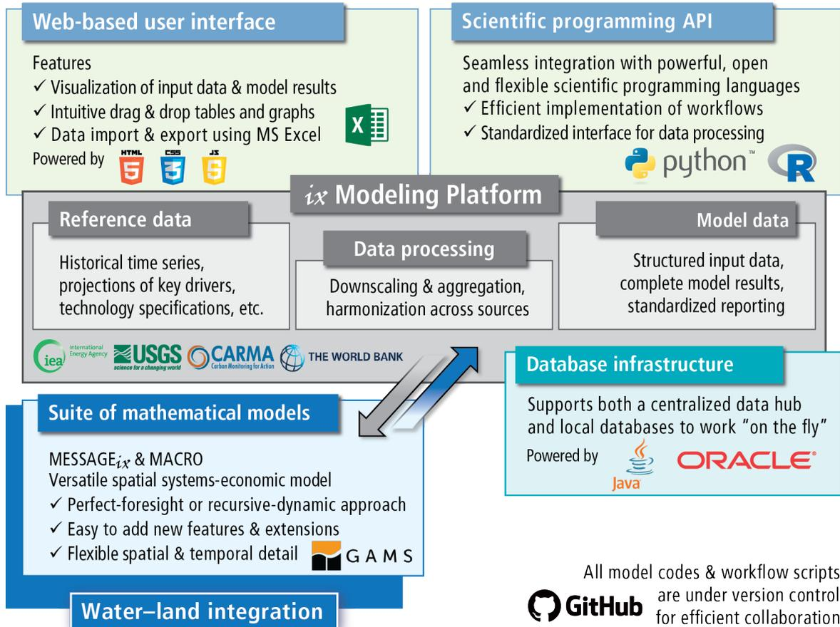
Fig. 1: Components and their interlinkages in the *ix modeling platform* (source [1]): web-based user interface, scientific programming interface, modeling platform, database backend, implementation of the MESSAGE<sub>ix</sub> mathematical model formulation.
