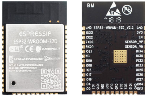
Fig. 2: ESP32-WROOM-32D module (front and back)
