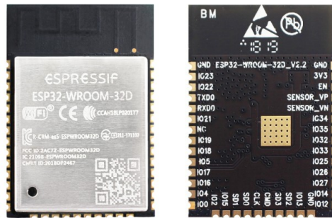
Fig. 2: ESP32-WROOM-32D module (front and back)
