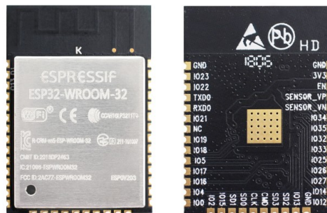
Fig. 1: ESP32-WROOM-32 module (front and back)
