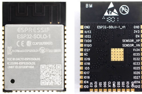
Fig. 4: ESP32-SOLO-1 module (front and back)
