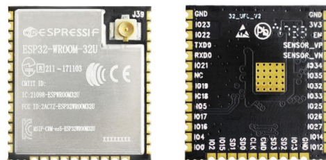
Fig. 3: ESP32-WROOM-32U module (front and back)
